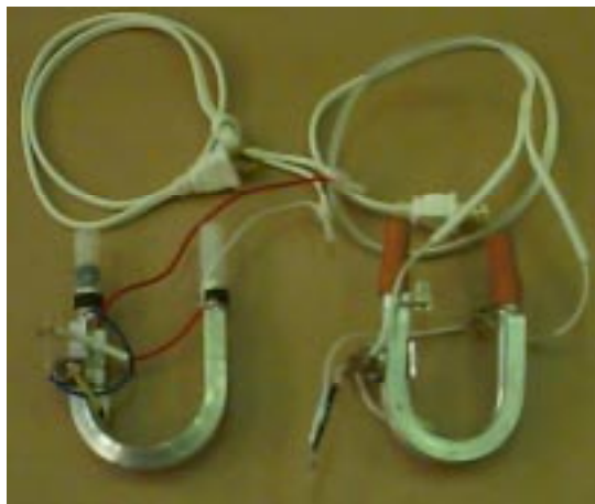
Figure 3.20 West Bend (left) and Mr. Coffee (right) electrical supply and electrical conversion modules present in the iced tea brewers.
