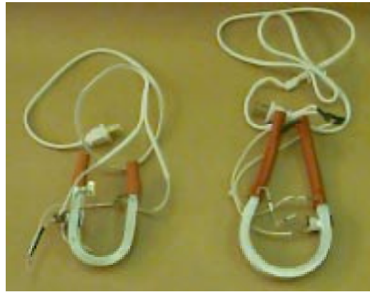
Figure 3.24 Mr. Coffee iced tea brewer (left) and coffee maker (right) electricity to thermal energy modules .
