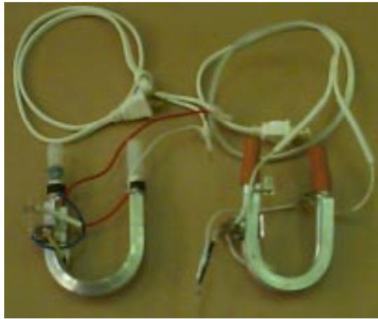
Figure 6.19 Examples of existing components that solve the electrical supply and electrical conversion modules for the iced tea brewer. These modules are used in iced tea brewers and coffee makers.
