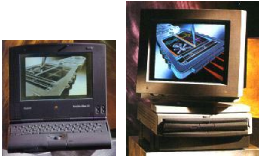
Figure 3.6 The Apple PowerBook Duo line of computers is an example of sectional modularity. The PowerBook Duo (left) can be used as a stand alone computer or can be used as the CPU section of the desktop system shown on the right. (Photo by Paul Franz-Moore.)
